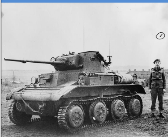
Tetrarch, Light Tank Mk.VII, A17 w/Littlejohn adapter fitted to 2-Pounder
