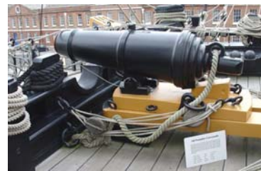
68-Pound Carronade (short, smoothbore, cast iron cannon, Carron Company, Falkirk, Scotland)
