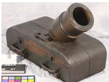
24 pounder (6") Coehorn Mortar Effective range: 20-1,200 yards (in theory) Total weight: 300 lbs (barrel 164 lbs)
