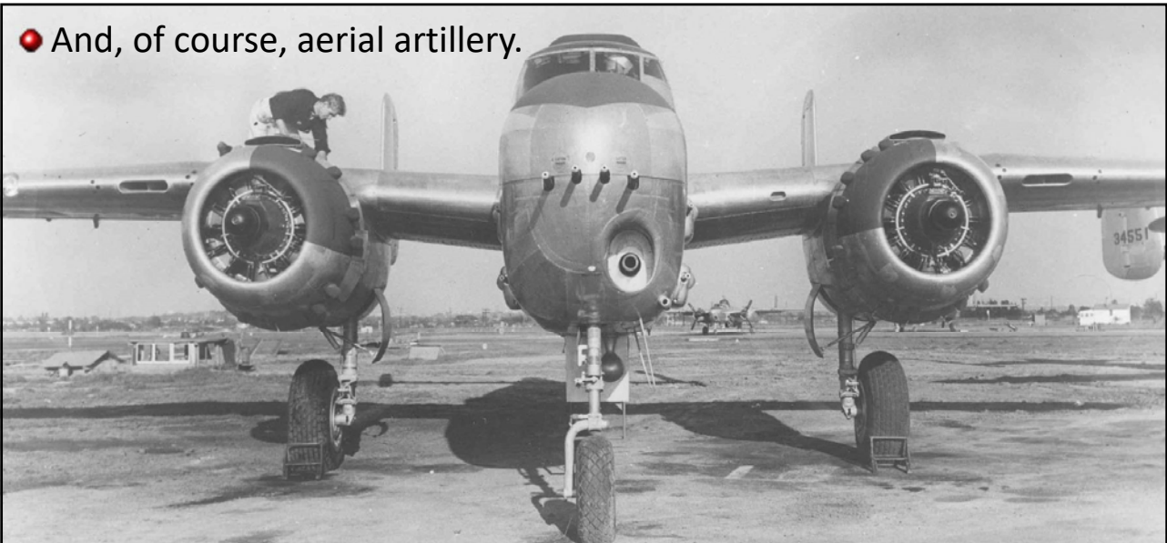
B-25H with 4x.50 calibre machine guns and a 75mm cannon, as modified by MAJ Pappy Gunn for use as an attack aircraft by the US Army Air Corps of SWAPA in New Guinea.
